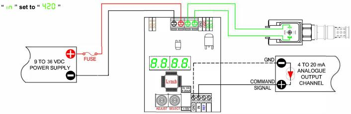
TWO WIRE TRANSMITTER INPUT CONNECTION
